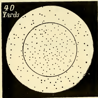
Pattern of the Cylinder Gun at 40 Yards.
